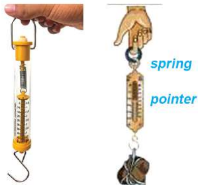
Figure 7.13: Measurement of weight by a spring balance
